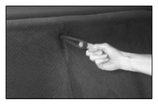
To fold down the rear seat, pull forward on the seat tab to unlatch the seatback.
